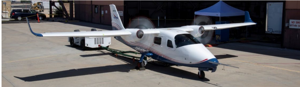
Figure 3 – X-57 in the Mod II configuration during a ground test.
