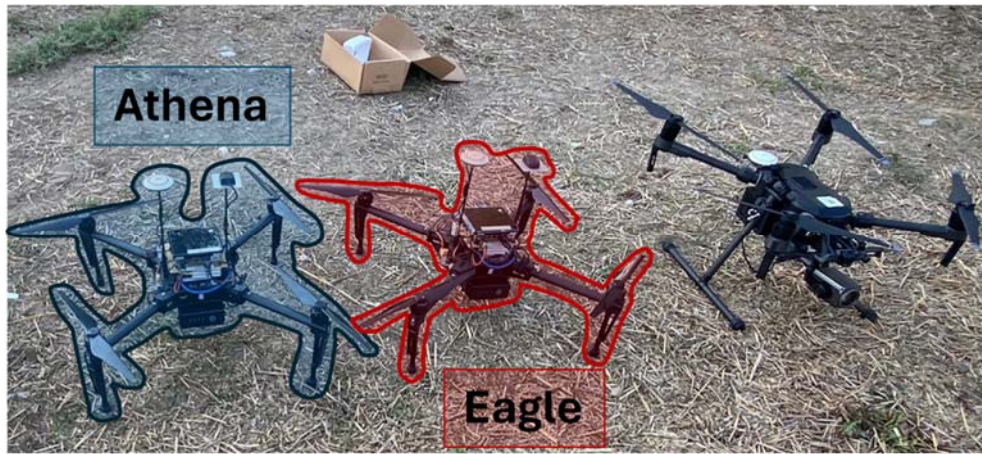
Figure 3 – Drones used during experimental tests. Drones used for the results discussed in this paper are highlighted in blue (ownership – Athena) and red (intruder – Eagle).
