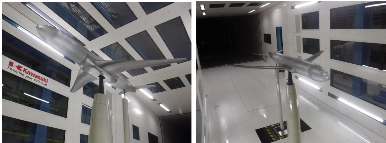
KHI CRM-HS with the strut support system
