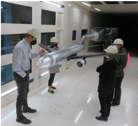
Figure 30– Model verification by the CRM-HL Ecosystem team in the 2 nd testing campaign
