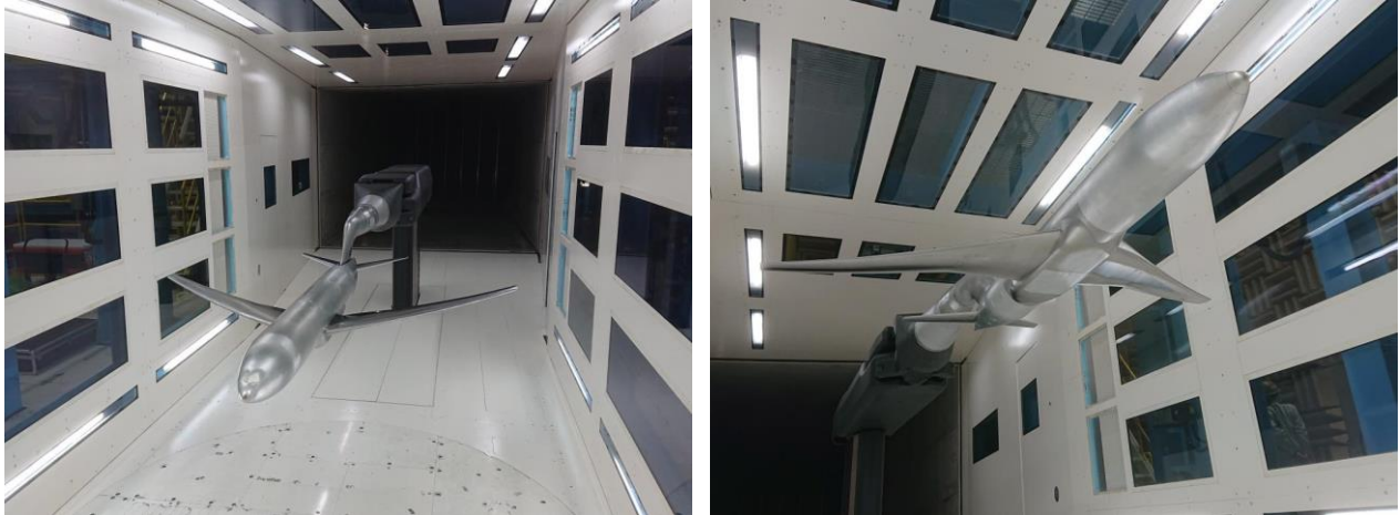
KHI CRM-HS with the sting support system
