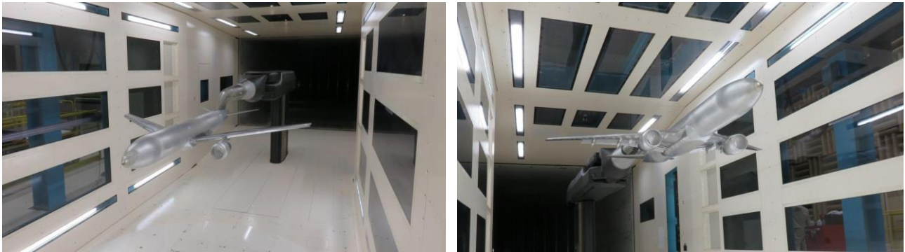
Figure 22– KHI-CRM-HL model at KLWT in 1 st testing campaign (Oct.2022)
