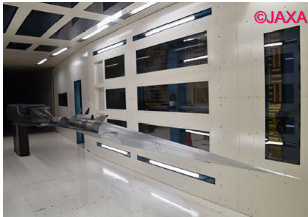
Test with the sting support in closed section [13]
