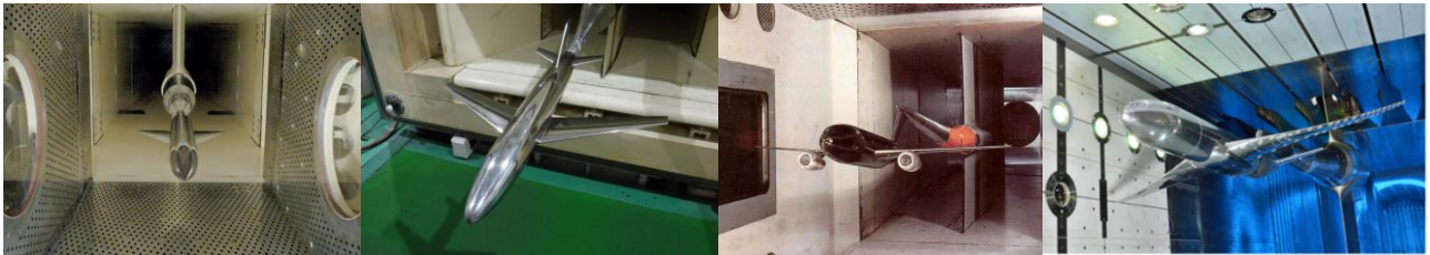
AGARD-B/C (1952-) ONERA-MX (1969-) DLR-F4/F6(198X-) [18] NASA-CRM (2008-) [12] Figure 14– KLWT Check model candidates (public shapes of check standard model)
