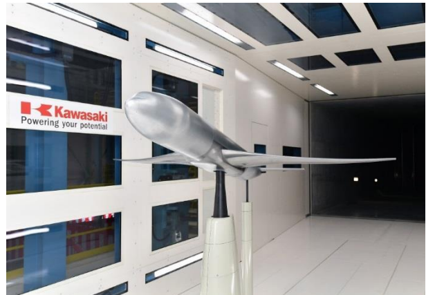
Test with the strut support in closed section
