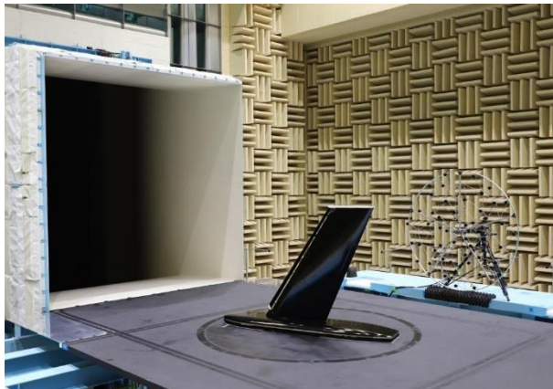
Acoustic test with half model [14-17]
