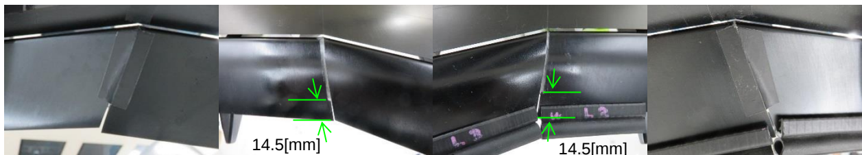
Gap seal configuration 1 (A64W001 - A64W006) (ONERA 1/19.5 style)
