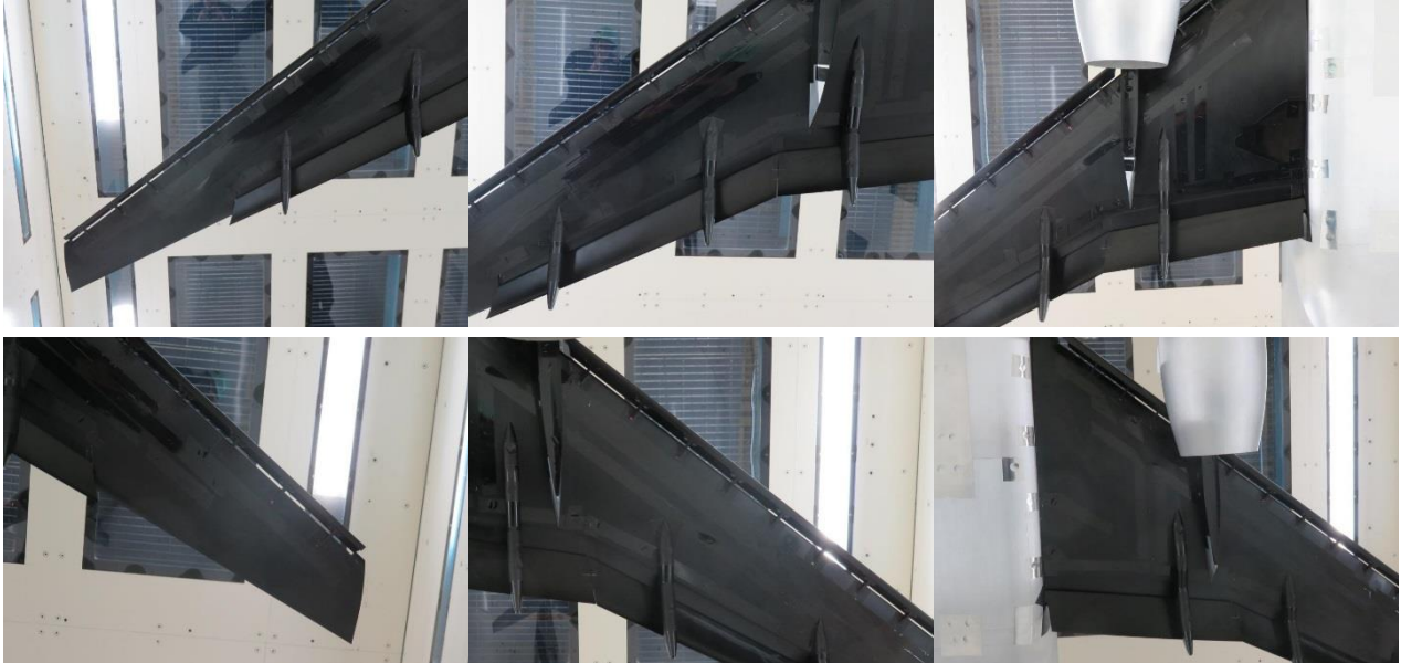
Figure 29– KHI CRM-HL model finish under wing
