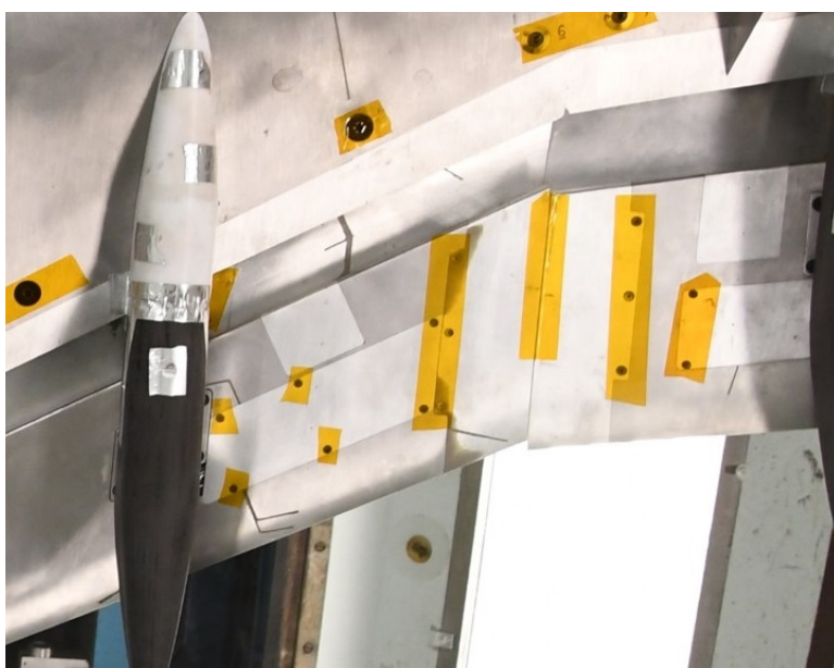
Figure 8 – Inboard to Outboard Flap Junction as tested in QinteiQ on the NASA 10% model
