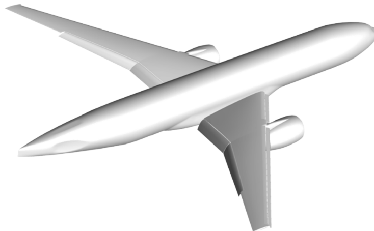
Figure 3 - Reference CRM-HL landing configuration.
