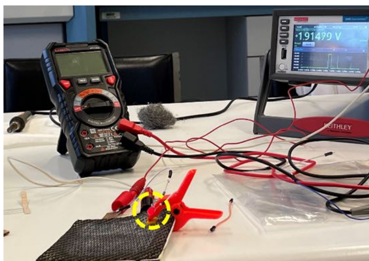
Figure 13 – LED connecting to SB current collectors confirming its functionality.
