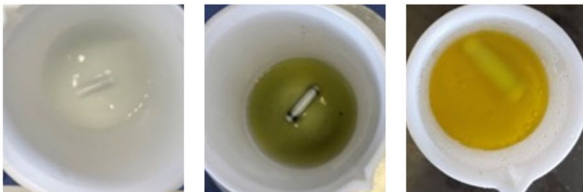
Figure 8 - Steps in the preparation of the solution chosen for CF tissue impregnation: solution of \text{HNO}_3 , \text{HCl} and \text{H}_2\text{SO}_4 (left), \text{LiFePO}_4 addition (center) and dissolution (right).
