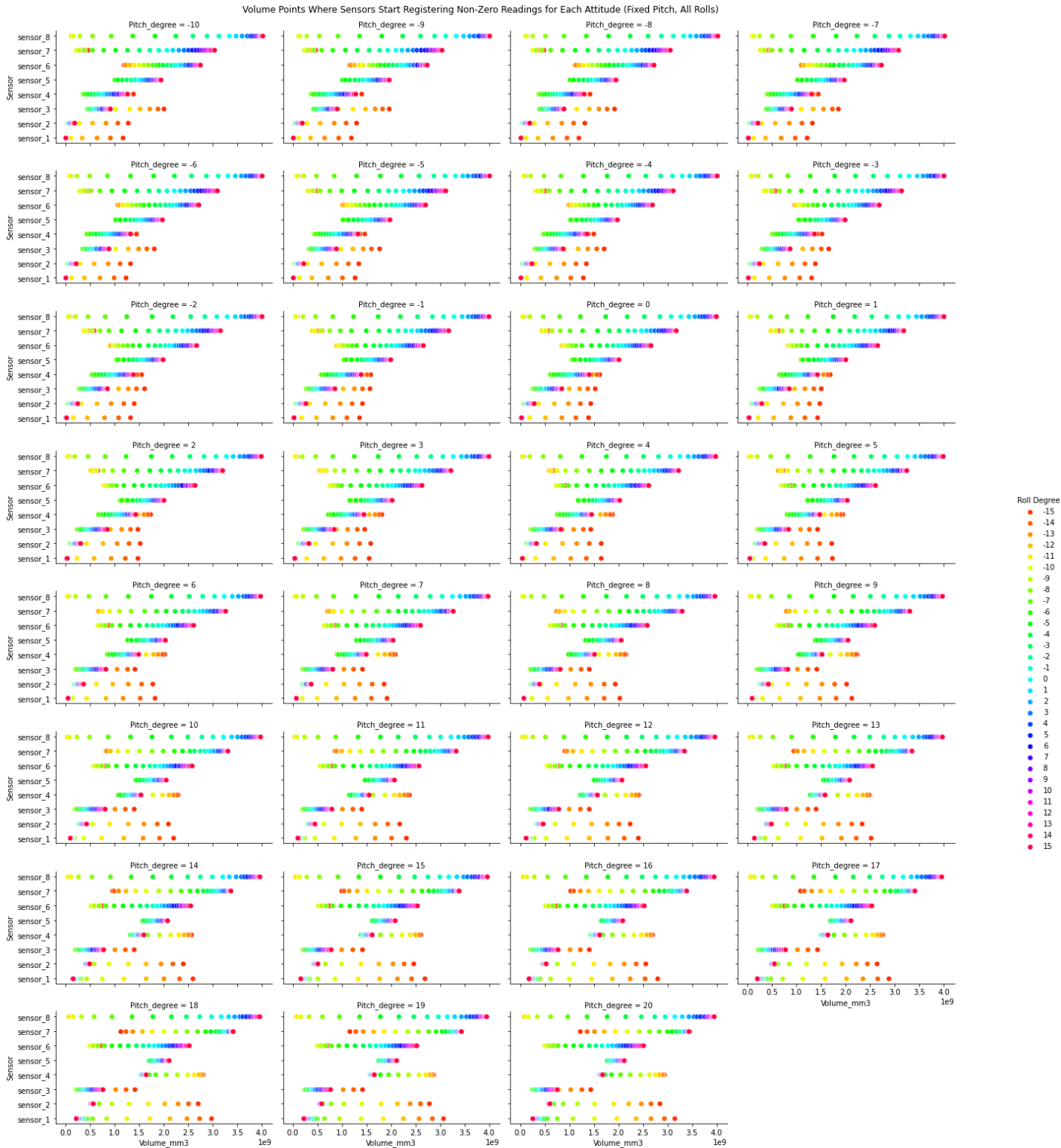
Figure 9 – Figure capturing where each sensor starts to measure in all attitudes.
