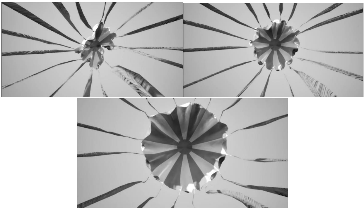
Figure 11 – Air force parachute inflation bottom view processed simulation data
