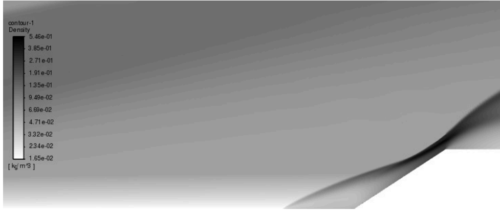
Figure 7 – Density gradient contour for k - \omega turbulence model
