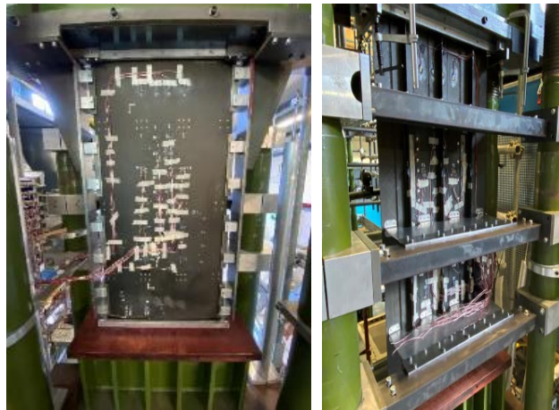
Figure 8. Test set up completed and ready to start fatigue cycling.
