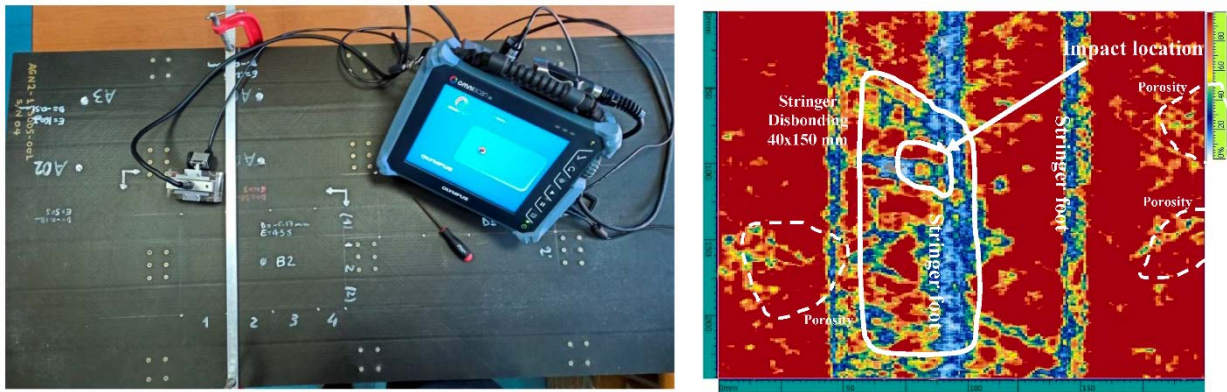
Figure 3 – NDI via phased array ultrasonic scanning.
