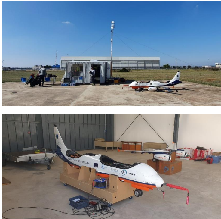
Figure 5: Photos of the SFD ready for operations on the GCS platform area (top) and in the hangar for maintenance operations (bottom)
