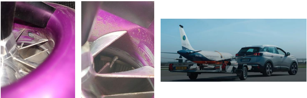
Figure 7: FOD on the SFD engines (left and middle) and operational solution to mitigate the risk (right)
