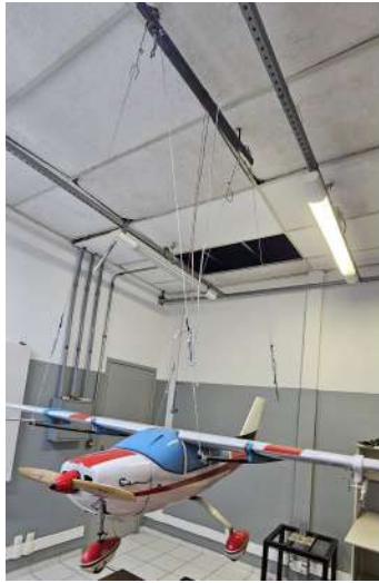
Figure 8 – Test conducted for the measurement of inertia in I_{xx} .
