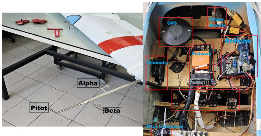
Figure 3 – Electronic system installed on the Cessna 177B subscale aircraft.
