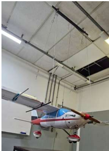
Figure 9 – Test conducted for the measurement of inertia in I_{yy} .
