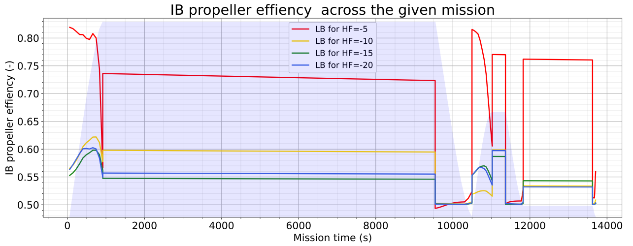
Figure 22 – Efficiency of the IB propellers across the mission profile and selected lower HF^* bounds.
