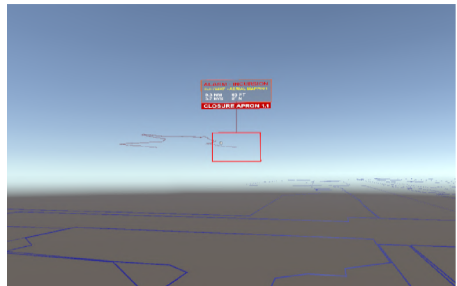
b) Visualisation in the simulation environment of the interface appearance during a drone intrusion inside the airport restricted area.
