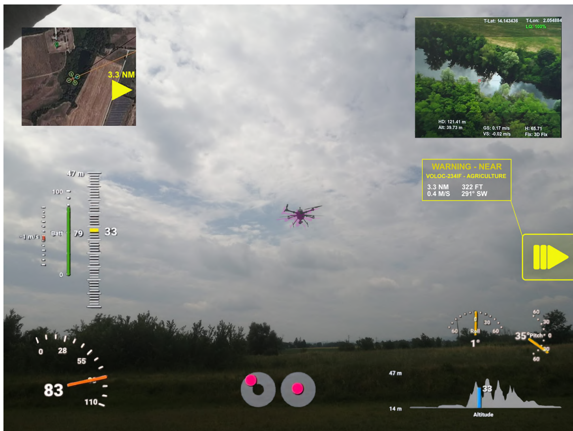
Figure 5 – Proposed design for the drone interface in a piloting scenario.
