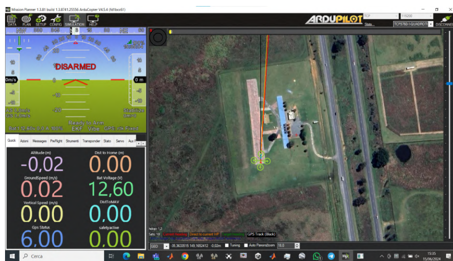
Figure 1 – A conventional head-down interface for drone piloting built on the ArduPilot Mission Planner open-source software.
