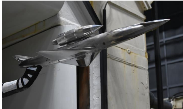
Figure 12 – CS-2 model installed on the pitch mechanism.
