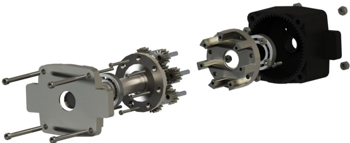
Figure 8 – Exploded view of the designed planetary gearbox.
