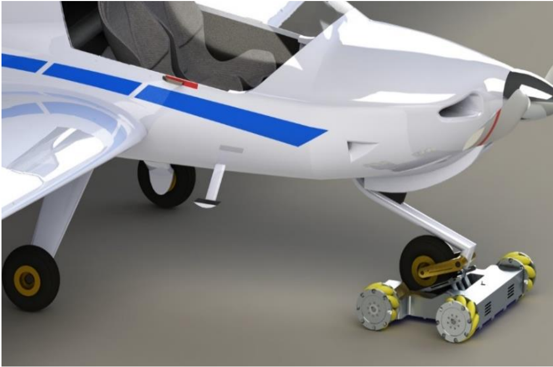
Figure 3 – The front landing gear of the Diamond DA-20 aircraft on the designed CRAWLER 01 tug.
