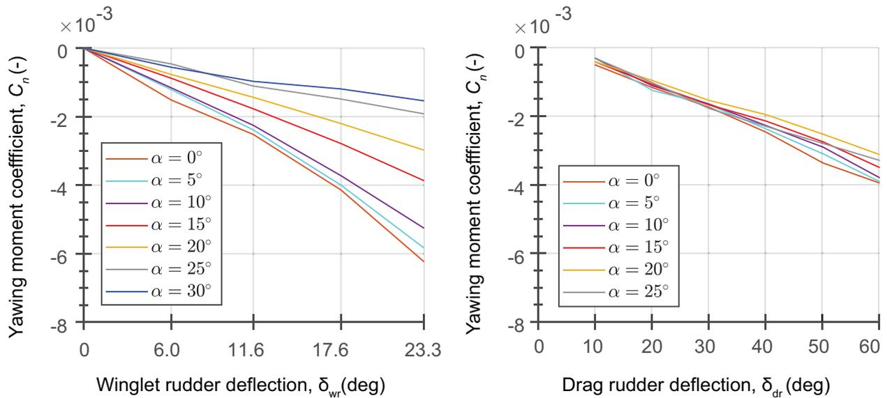
Figure 9 – Yawing moment coefficient due to deflection of both winglets (left) and due to deflection of a 5%-span drag rudder (right).  $Re = 1.1 \cdot 10^6$
