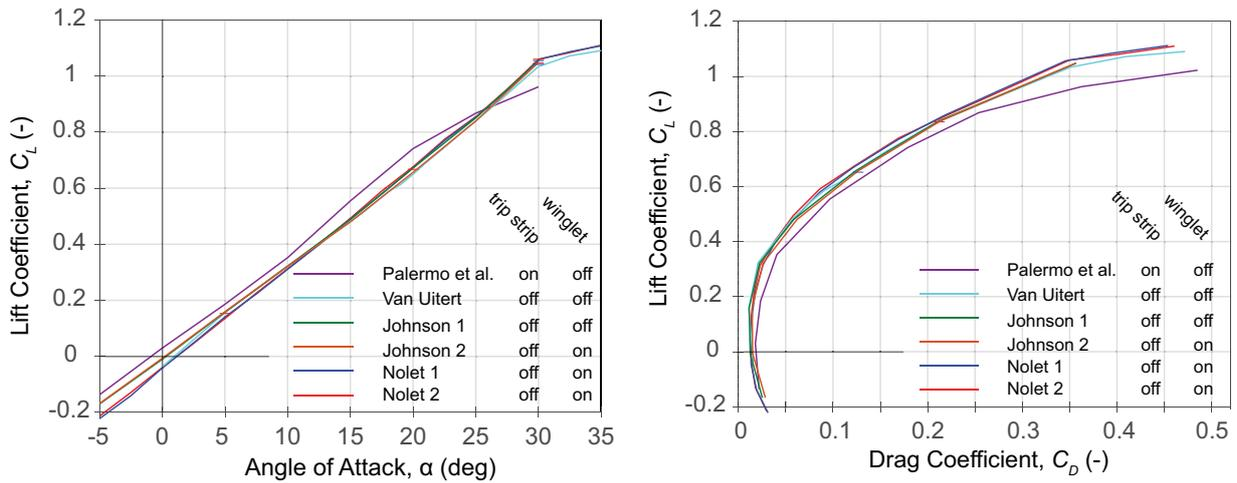
Figure 7 – Comparison of lift curve (left) and drag polar (right) results to previous studies. The Reynolds number is between 1.0 and 1.1 million for all experiments.
