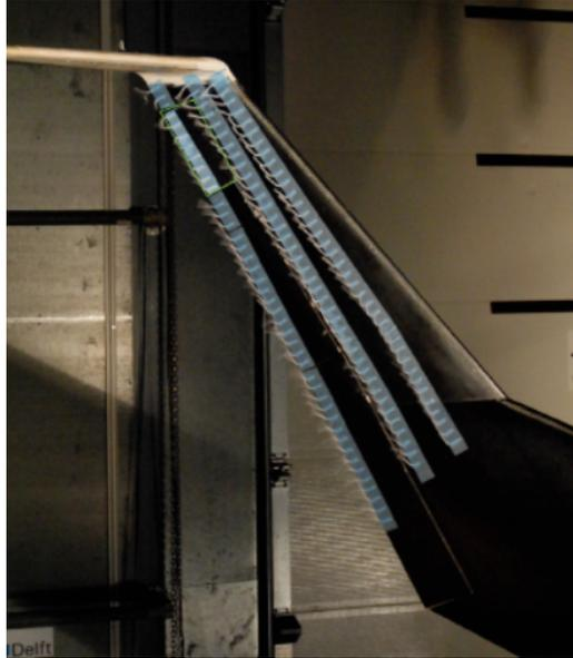
Figure 6 – Experimental setup with 40-degree deflection of upper drag-rudder panel and tufts.
