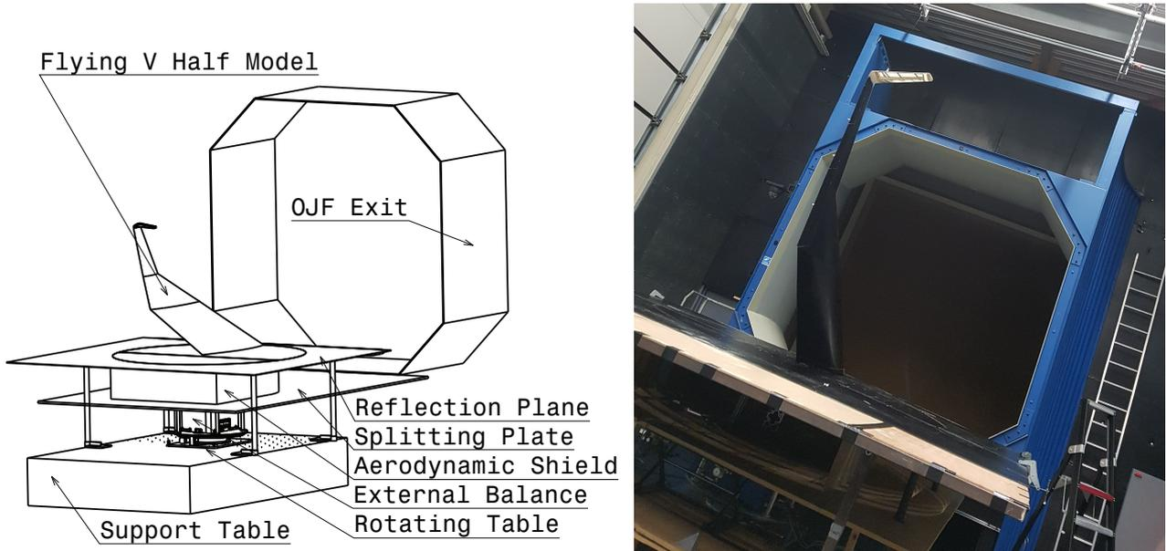
Figure 2 – Flying V half model in the Open Jet Facility (OJF) of TU Delft. Schematic (left) and photograph (right). The span of the half model is 1.5m. This drawing and image previously appeared in Ref. [6].
