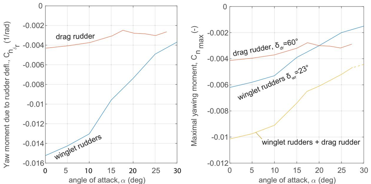
Figure 10 – Yawing moment derivative with rudder deflection (left) and yawing moment generated at maximal tested rudder deflection (right). Results for a 5%-span drag rudder.  $Re = 1.1 \cdot 10^6$
