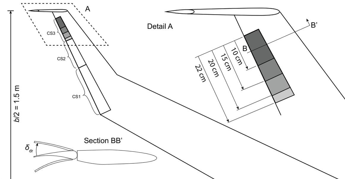
Figure 5 – Design of the drag rudders on the port-side wing. The most outboard control surface (CS3) mounts four drag rudders of various lengths. Modified from Ref. [6].
