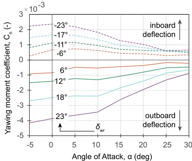
Figure 8 – Yawing moment variations with angle of attack for port-side-wing winglet rudder deflections ranging from -23 degrees to +23 degrees.  $Re = 1.1 \cdot 10^6$
