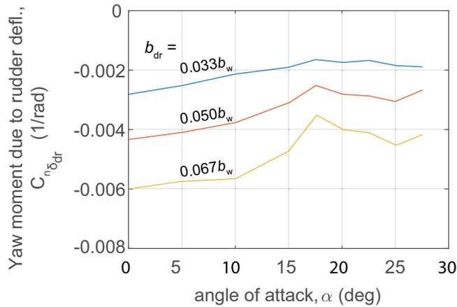
Figure 11 – Drag rudder effectiveness as a function of the drag rudder span ( $b_{dr}$ ). Experimental results at  $Re = 1.1 \cdot 10^6$ . Drag rudders according to layout in Figure 5.
