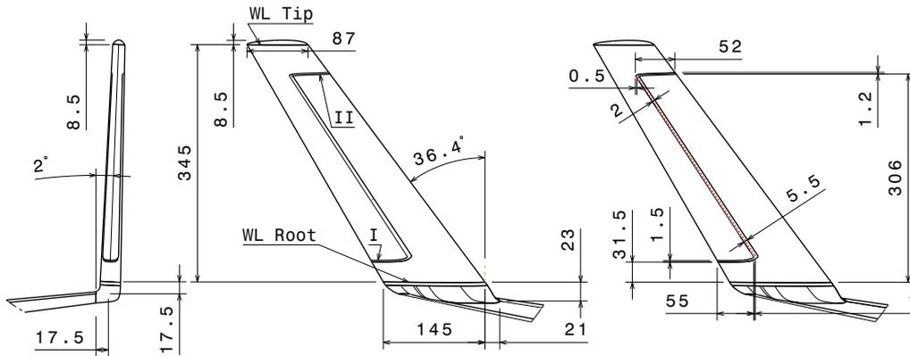
Figure 4 – Dimensions of the winglet (WL) and rudder [6]
