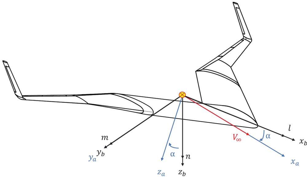
Figure 3 – Body-fixed and aerodynamic reference frames for zero sideslip. The rolling, pitching, and yawing moments are indicated with  $l$ ,  $m$ , and  $n$ , respectively. This image previously appeared in Ref. [6].
