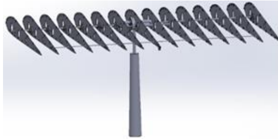
Figure 2-Internal structure of wind tunnel model.
