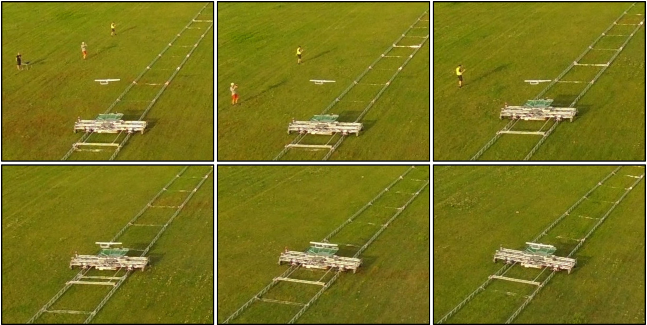
Figure 6 – Landing sequence of a drone on the GROLAS system. The time interval between the images is 1 sec.
