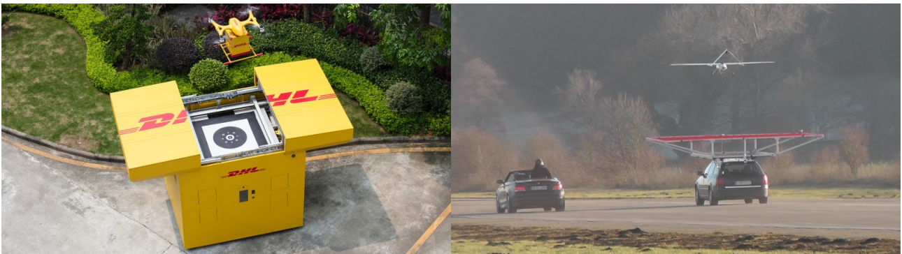
Figure 4 – Automated eVTOL launch-&-landing pad of the DHL parcelcopter (left). DLR landing a fixed-wing UAV on a moving platform (right).
