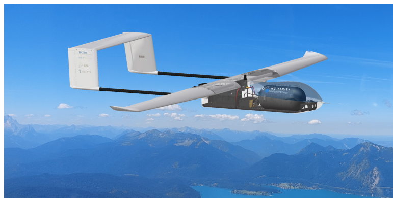
Figure 3 – The H2 FINITY concept of a silent long-range drone, powered by a H 2 -fuel cell and electric propulsion
