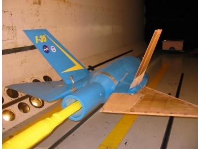
Figure 12 Scaled F-35 flutter model wind tunnel test[37]
