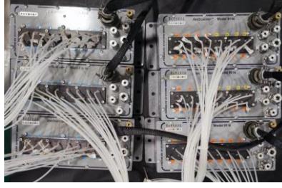
Figure 2 The PSI electronic pressure scanning valves.
