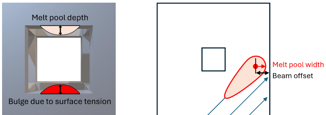
Figure 11 – Images of contributions for the geometrical difference in the fabricated lattice structures due to the meltpool depth/surface tension (left) and the meltpool width and beam offset (right).
