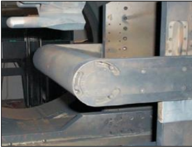
Figure 2- HEG Cylinder Test Geometry [2]
