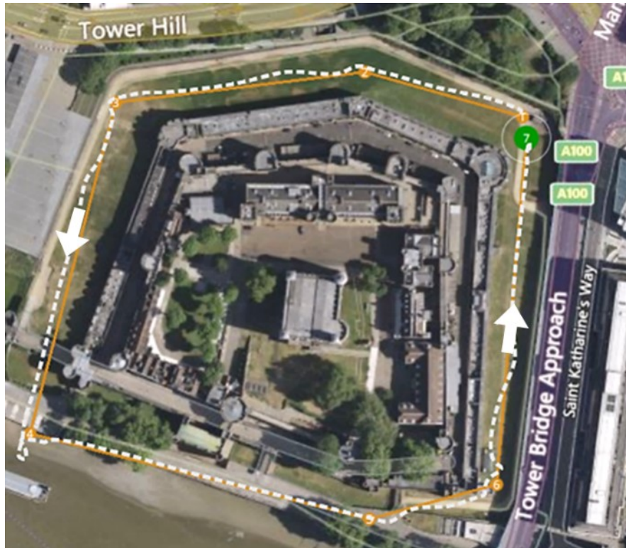
Figure 8: Trajectory waypoints specified in QGroundControl (orange) and overlaid the path followed in simulation (white).
