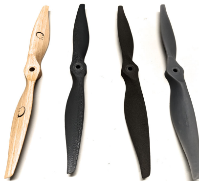
Figure 3 – The propellers tested in this investigation. From left to right: original wooden propeller, FDM, SLS and SLA-manufactured versions.
