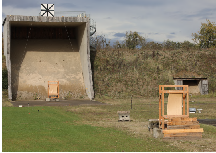
Figure 5 – Paper frames at the entrance and exit of the acoustic measurement zone.
