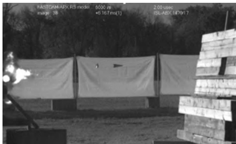
Figure 2 – Snapshot of the projectile in flight, close to the sabot catchers.
