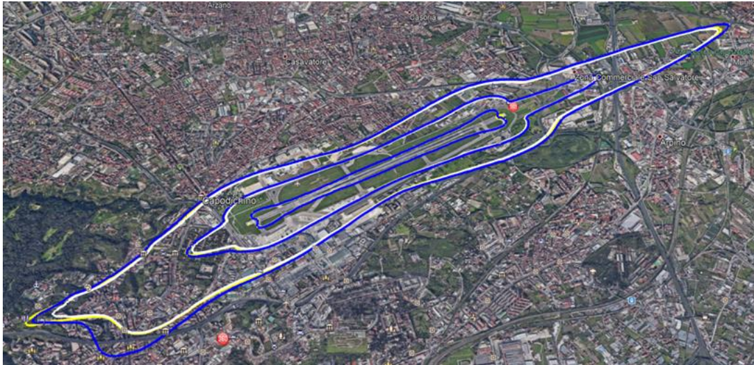
Figure 5 – Example of actual noise contours at Capodichino airport
