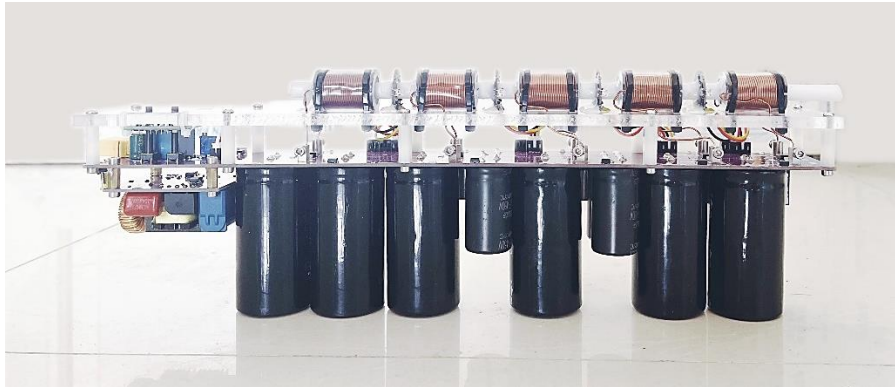
Figure 13 – A scaled 5-stage electromagnetic coilgun.
