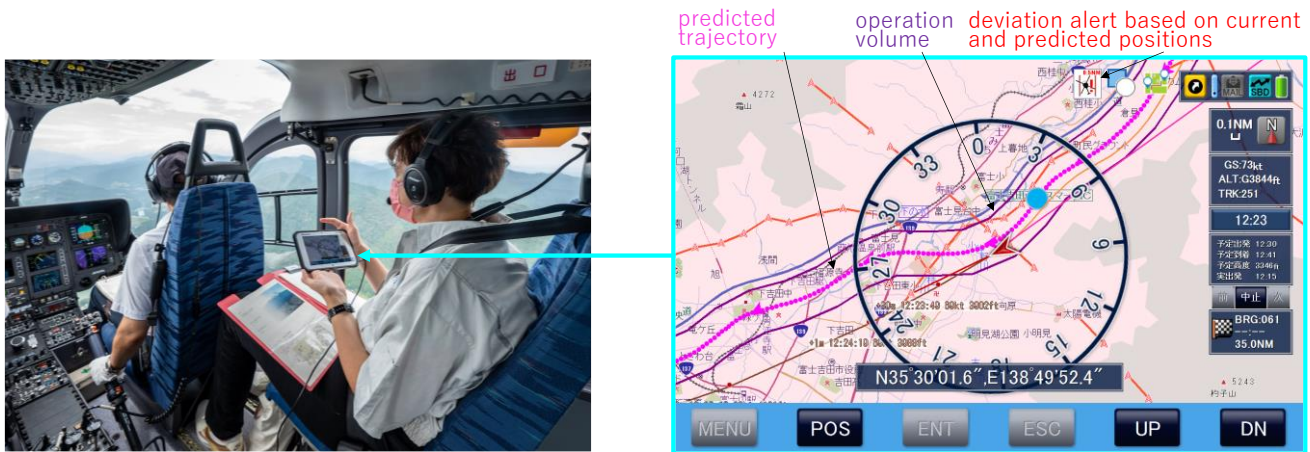
Figure 8 - D-PAS display with operation volume and predicted lateral trajectory.
