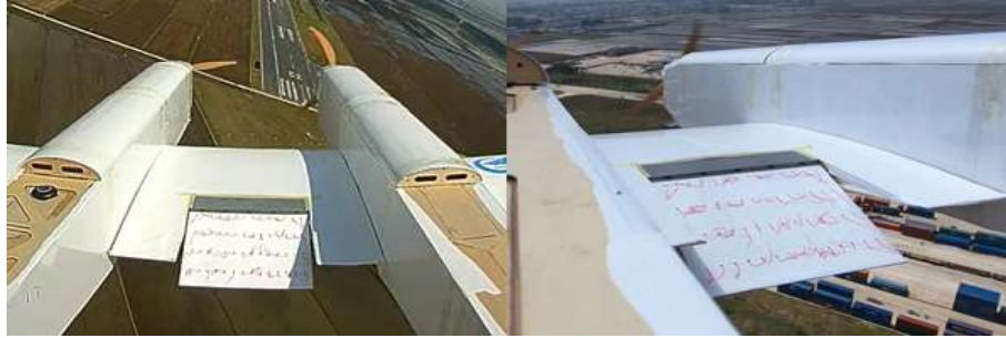
(b) The level-flight state with flap opened and jet closed
