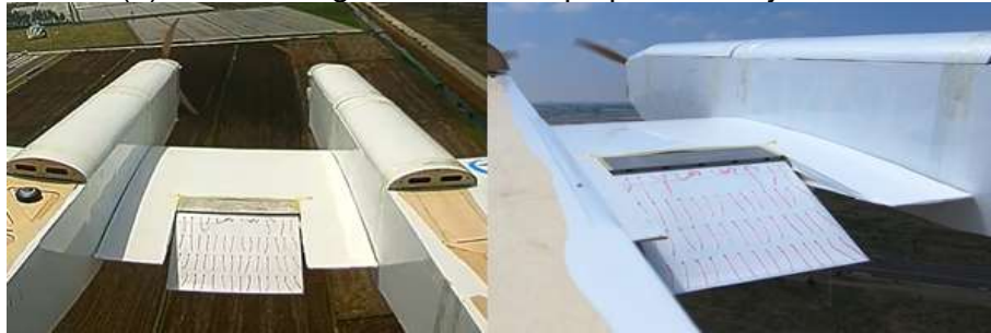
(c) The level-flight state with flap opened and jet opened
