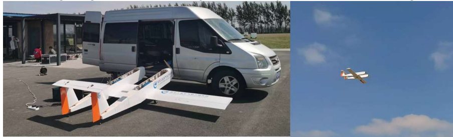
Figure 9 – The dual-fuselage flight platform in ground preparation and air flight.
