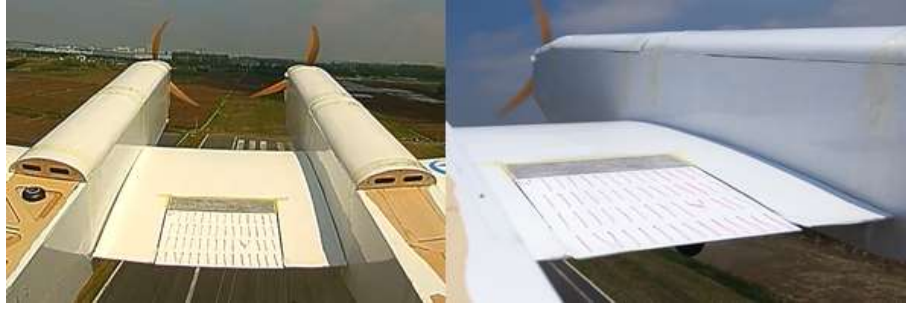
(a) The level-flight state with flap retracted and jet closed
