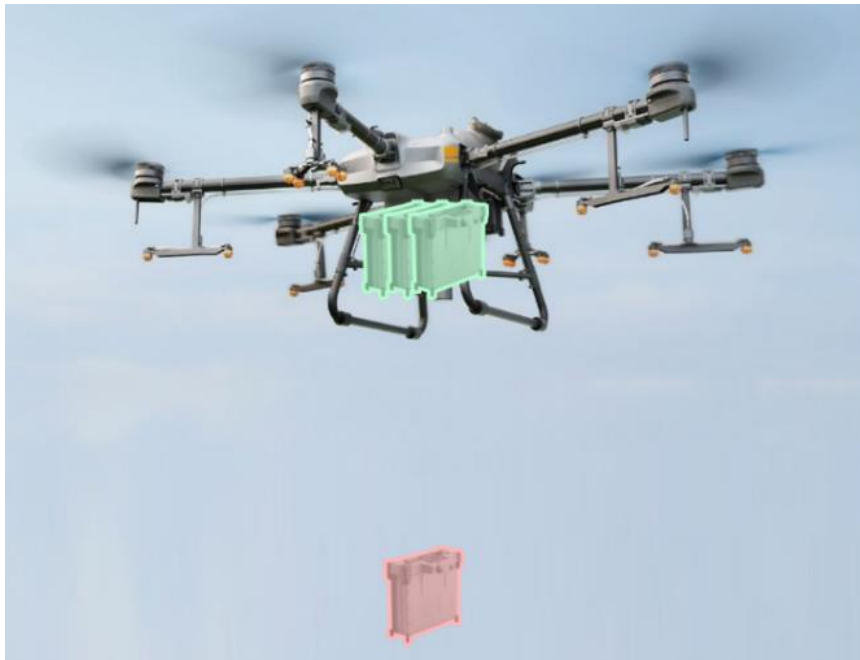
Figure 1 – Conceptual view of battery multi-stage separation technology (green: charged batteries, red: discharged battery)
