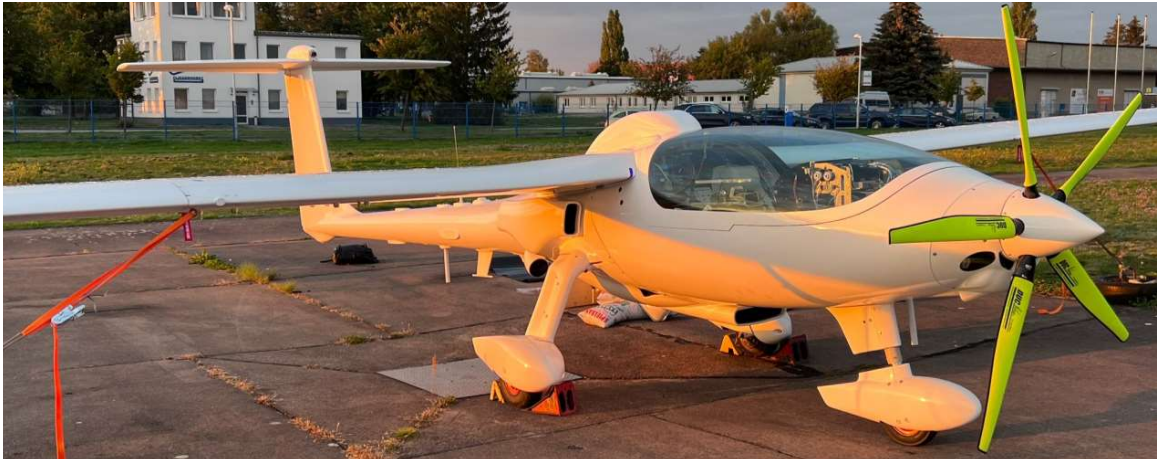
Figure 1 – HAPS flight demonstrator H001 by Stemme Belgium under development
