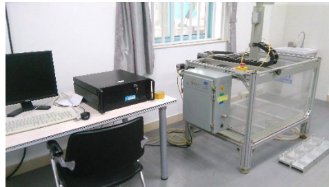
Figure 5 UPK-T36 ultrasonic immersion C-scan system
