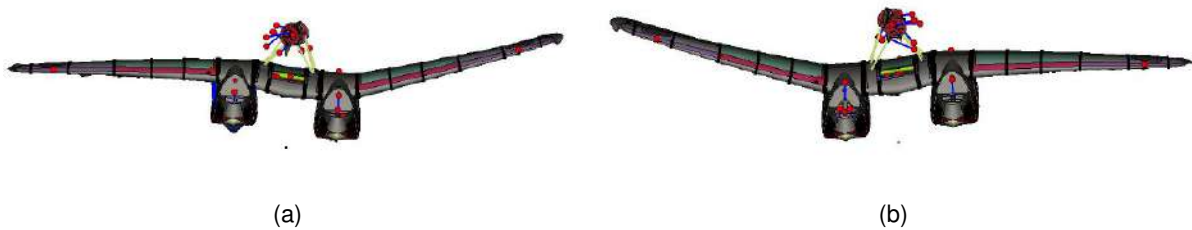
Figure 10 – Frequency: 43.1 Hz - II Bending
