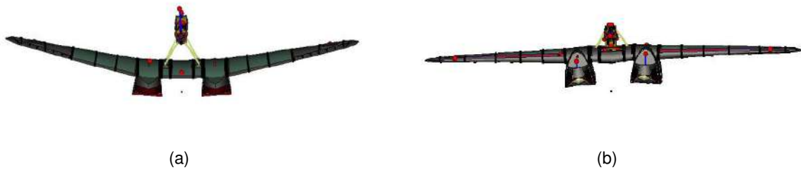
Figure 9 – Frequency: 20.7 Hz - I Bending
