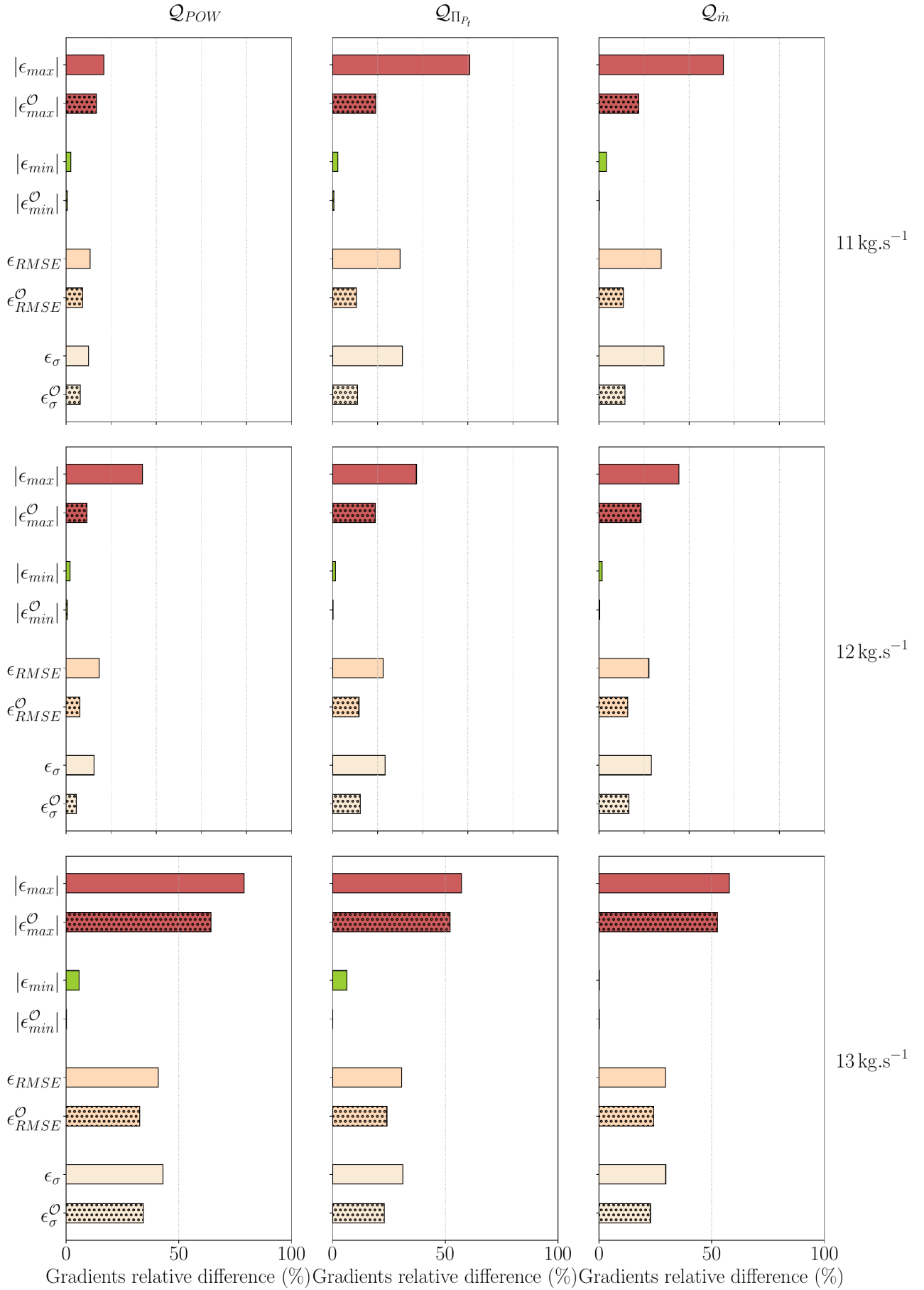
Figure 9 – Error metrics between ABFM and adjoint blade-resolved gradient evaluations for the three studied QoIs (columns) and the three studied operating conditions at \dot{m} = 11, 12 and 13 \text{ kg.s}^{-1} (rows) for the rotor shape gradients. Dots-filled bars represent the error metrics relative to the maximum of the blade-resolved gradient values observed.
