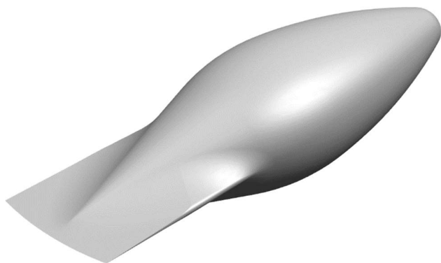
Figure 8 - A body specialised in favour of mass and drag with a trailing edge, which serves to induce circulation over the body and to bring a neutral point onto the body. Such a stable lifting body can be inflated to any size while retaining its flight mechanic properties.
