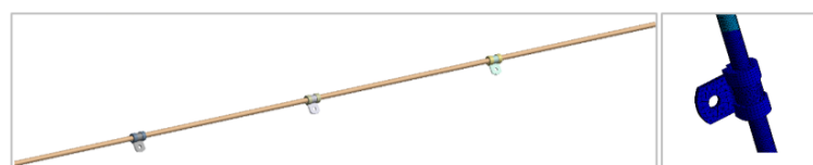
Figure 8 – Evenly distributed clamps supporting a pipe.
