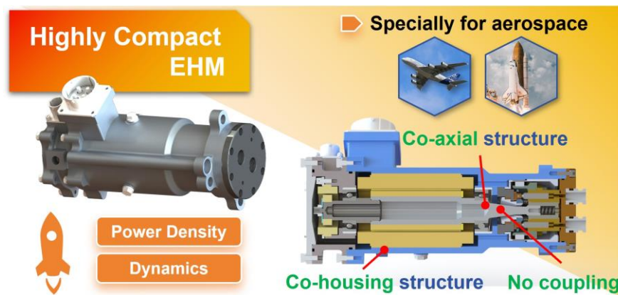
Figure 3 – The application scenario and structural characteristics of the EHM
