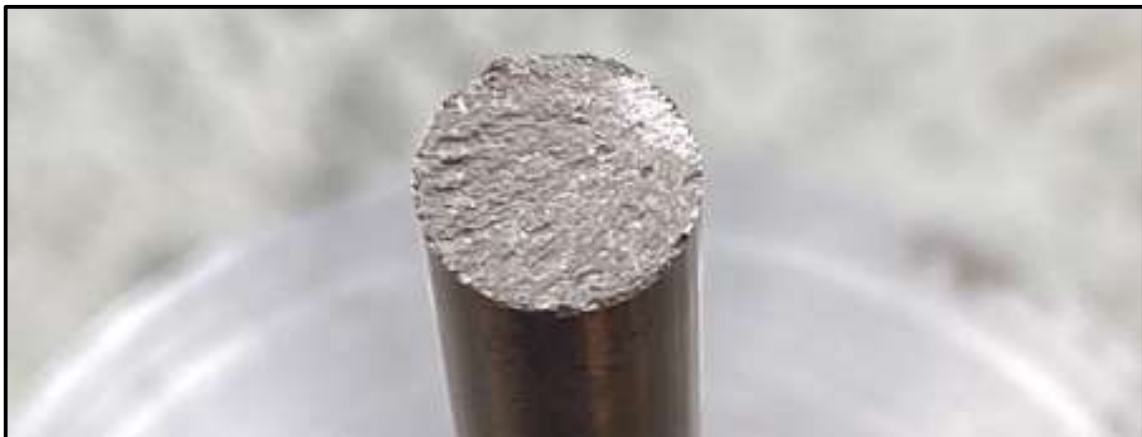
Figure 4 – Fractured surface of Specimen 18
