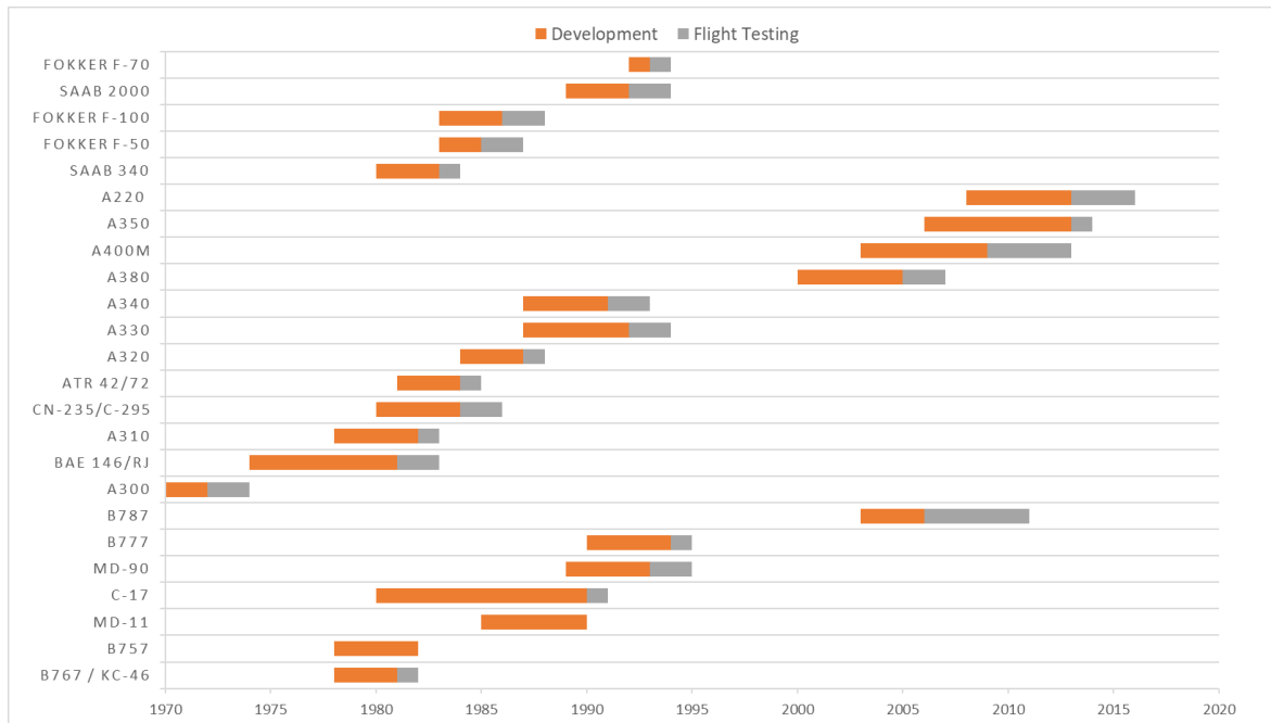
Figure 4 Development times of civil aircraft within the CS-25 category, from program start to first delivery
