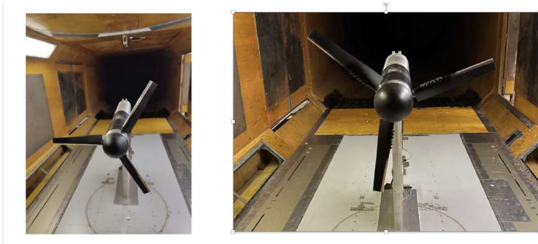
Figure 4 – Propeller test rig in the Cranfield University 8x6 Wind Tunnel.
