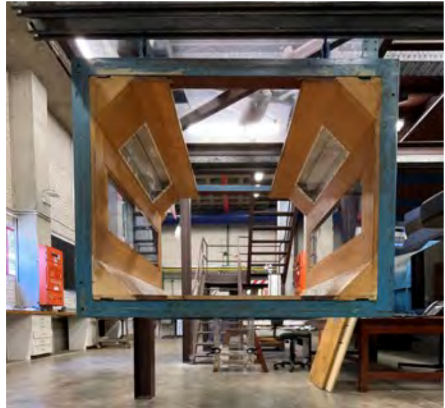
Figure 5 – The University of Sydney 4 ft \times 3 ft wind tunnel test section - front profile.
