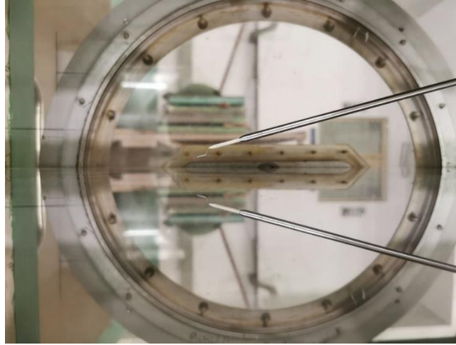
Figure 6 – Flat plate and the Dantec 55P15 boundary layer type probe. Notice the mirror-like appearance of the flat plate.
