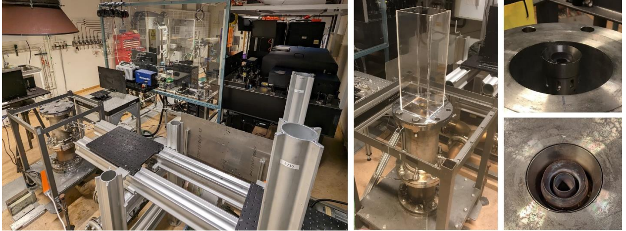
Figure 2 – Atmospheric combustion rig of Lund University, Division of Combustion Physics and integrated TARS burner.
