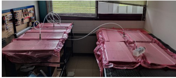
Figure 7 – Vacuum bagging for the wings.
