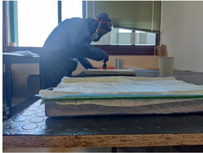
Figure 5 – Composite hand lay-up technique.
