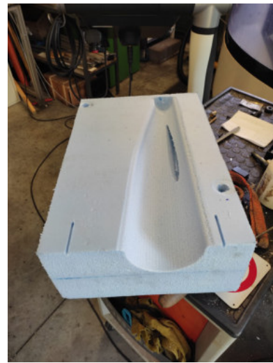
Figure 6 – XPS mould for the fuselage during (left) and after (right) the CNC machining.
