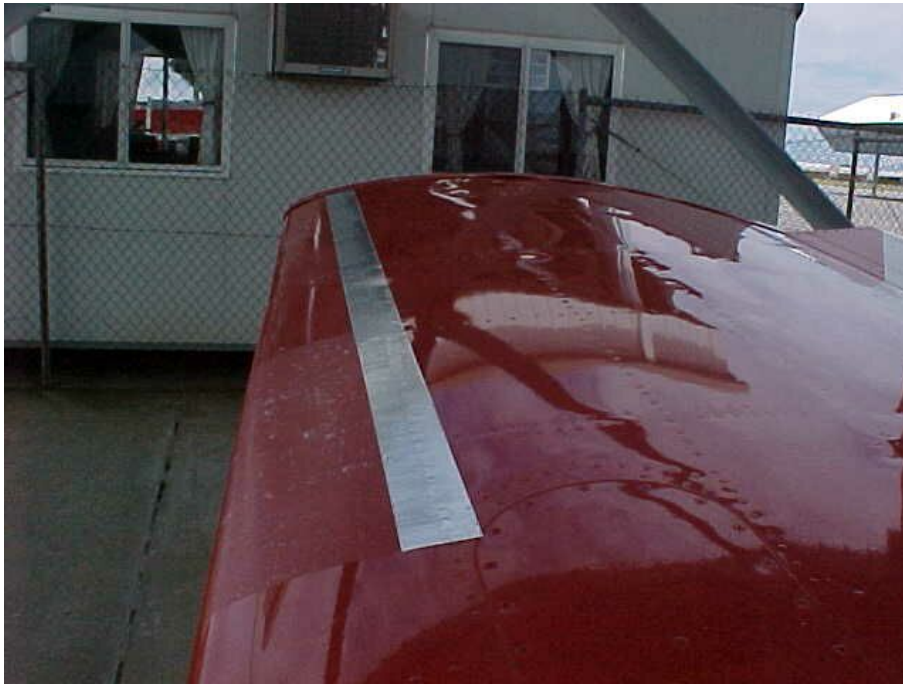
Figure 2 – Simulation of a paint step on the wing leading edge by aluminium tape
