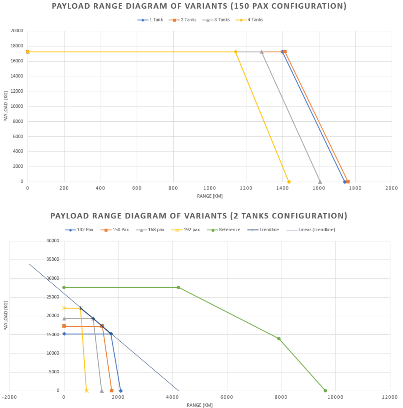
Figure 11 – (Top) Variation of Payload Range Diagram for PAX capacity (132, 150, 168, and 192 PAX) in 2 tank configurations and (Bottom) Variation with fixed PAX capacity (150 PAX) in reference to Airbus A320neo
