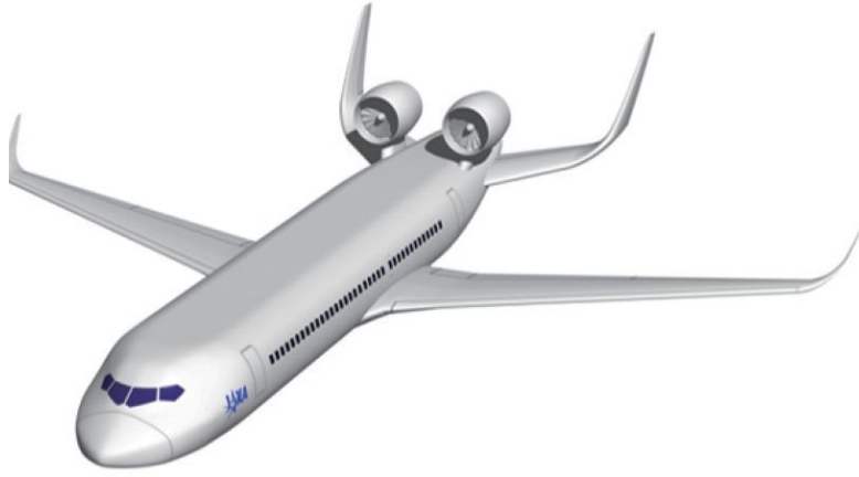
Figure 1 – Wide fuselage fuel-efficient, low-noise conceptual aircraft, HELNA, in the baseline configuration.
