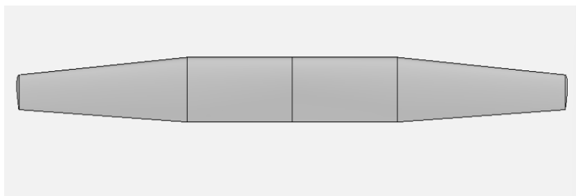
Figure 5 – Typical wing planform for regional turboprop applications assumed in the aerodynamic investigation.
