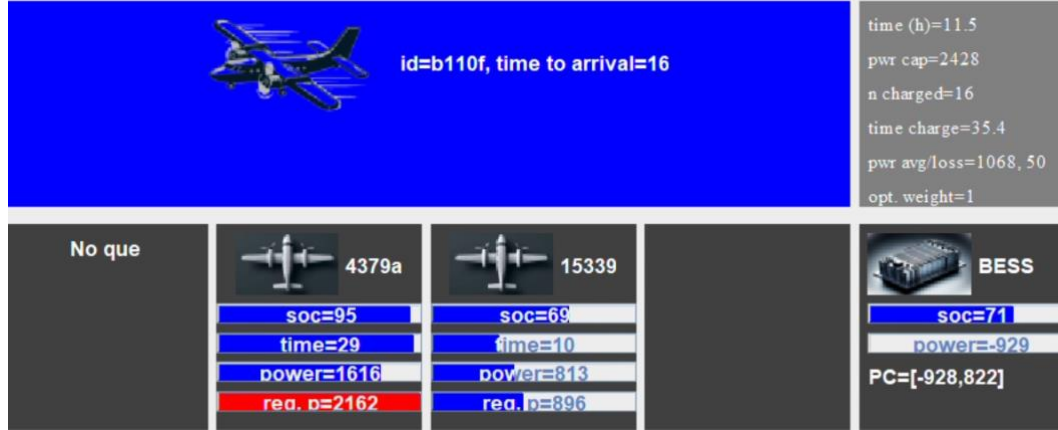
Figure 4 – Airport state 2. Two aircraft being charged simultaneously, sharing a reduced total system power capacity compared to airport state 1 in Figure 3. A failure state is observed with the current system settings.
